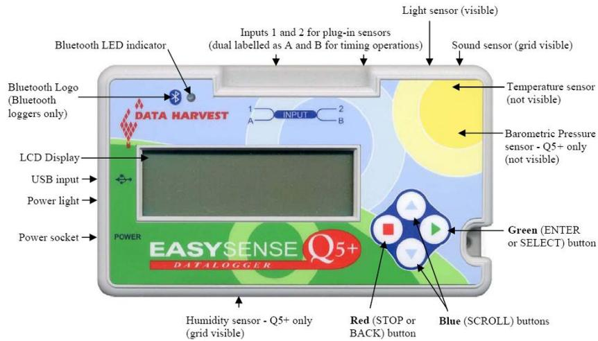
2. Plug the sensors into the inputs 1 and 2 slot.
